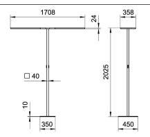
LED Light source Work equipment Electronic ballast DALI **Connected load** 220 - 240 V; AC; 50 Hz; 60 Hz **Power consumption** ca. 210 W; 214 W
