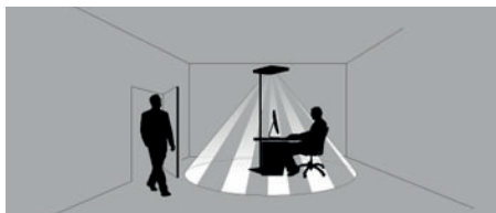
Fig. 9: Detection range of the PIR sensor.
