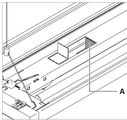
Fig. 5: Bend metal strap A downwards.
