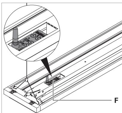
Fig. 7: Wireless module in a 2-lamp TYCOON suspended luminaire.
