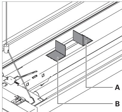
Fig. 4: Bend the half of the metal straps upwards.
