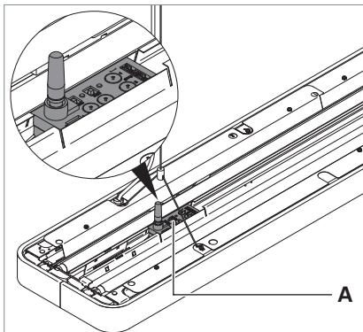
Fig. 3: Wireless module in a 2-lamp ATARO suspended luminaire.
