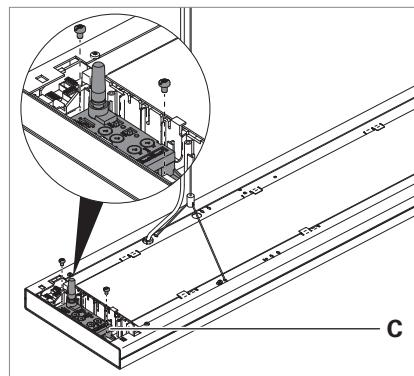
Fig. 2: Wireless module in a LAVIGO suspended luminaire.
